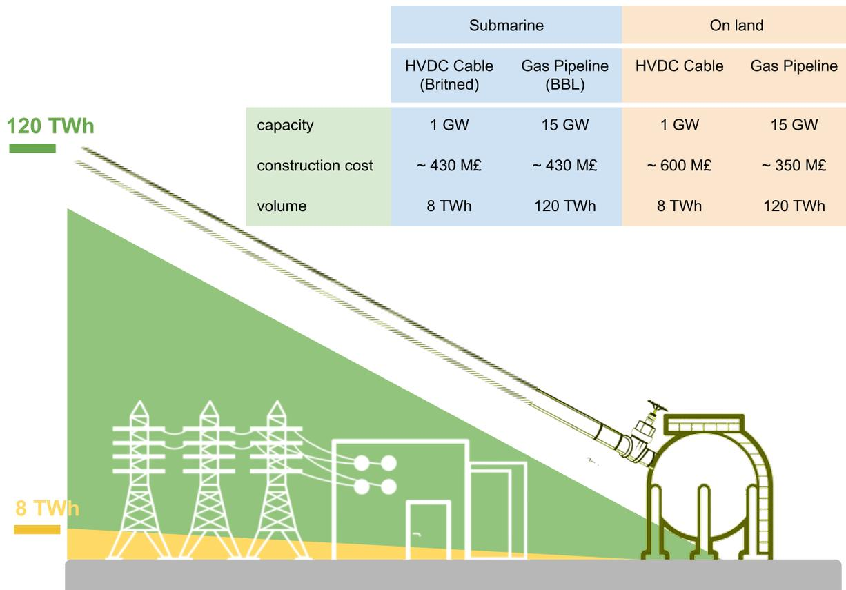
**REMARK:** BritNed is a 1 GW HVDC submarine power cable between the Isle of Grain in Kent in the UK and Maasvlakte in Rotterdam in the Netherlands. The BBL Pipeline (Balgzand Bacton Line, BBL) is a natural gas inter-connector between the Netherlands and the United Kingdom. The land deployment examples for electricity and gas pipeline are based on £/km standard price level back-of-the-envelope calculations.
